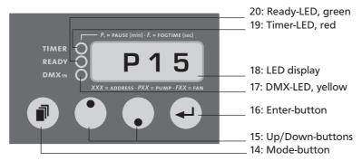
Fig. 1: Display shown at adjusting the pump output
