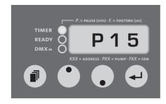
Adjusting of the output/pump in steps of 1% (1-99%)
